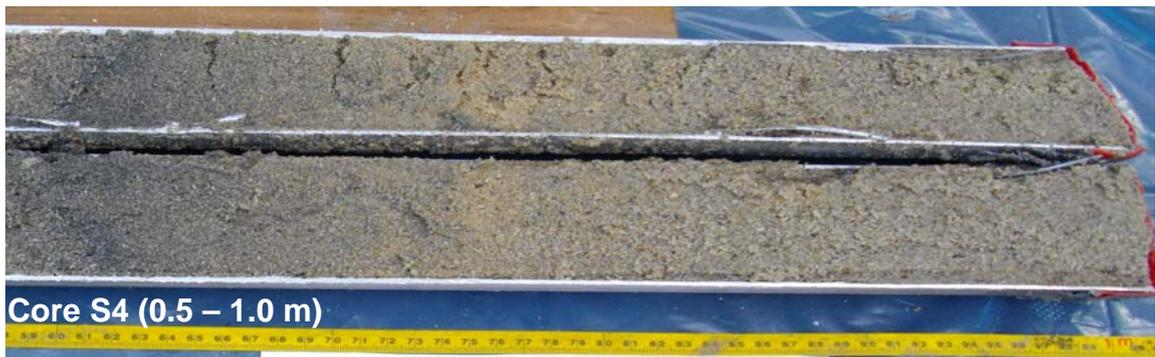
**Plate 2 Interbedded fine to coarse grained grey/brown sand and silty sand typical of the sediments retrieved from existing channel areas (ie. Cores S1, S2, S8 (at depth) and S9 – S10)**
